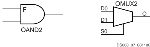
Figure 7: AND and MUX Symbols in Spartan-XL IOB
